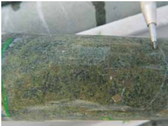
Late pyrite mineralisation in DDH1-9, in meta-basalt with epidote and chlorite alteration
