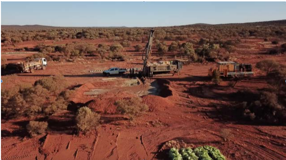
Figure 1: RC Drilling at Wodger Prospect
