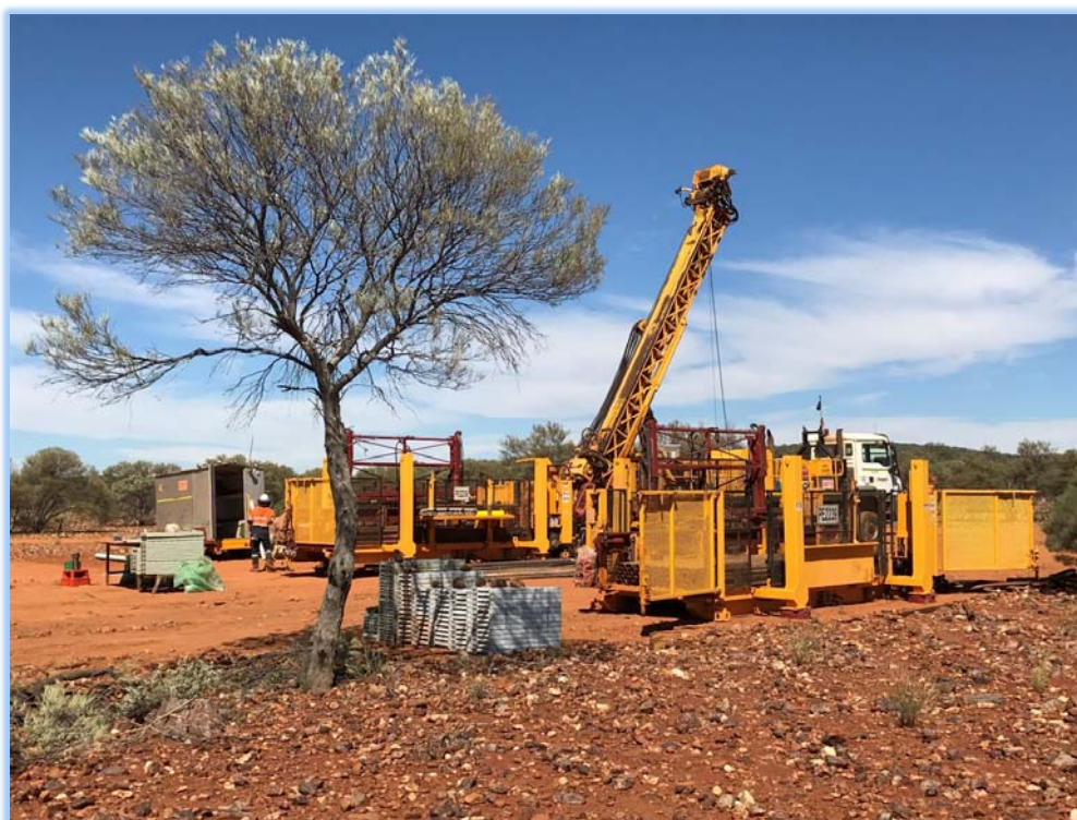
Figure 1: Diamond drill rig at Wodger
